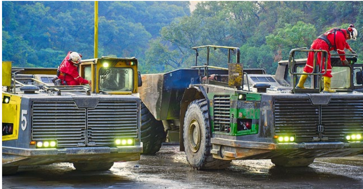
Inspecting low-profile trucks, Tizapa mining unit
