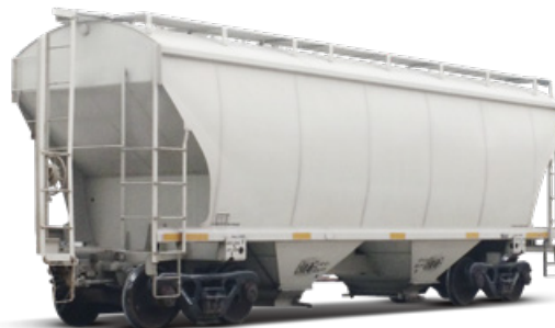
Granel en tolva de ferrocarril (Bulk in rail hopper car)
